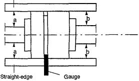
Fig. 10 - Aligning the coupling with the help of a gauge and a straight-edge
