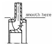
Fig. 18 Smoothing out the throttling sections on the impellers, see fig. 18a.
