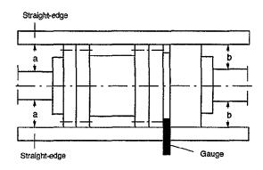
Fig. 11 - Aligning a spacer-type coupling
