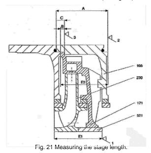
If machining of the stage sleeve is required, it should be shortened at both end faces in one operation on the machine tool. The permissible end face whobble (deviation from plane parallelism) is  $5 \,\mu$ m (micron meter).
