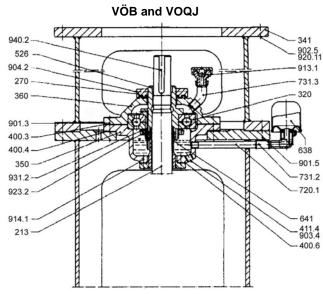
Fig. 07 Construction of support bearing VÖB (deep groove ball bearing and VÖQJ (four point contact bearing).
