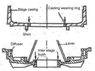
Fig. 02 Renewing the casing wear rings and stage bushes
