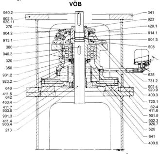
Fig. 08 Construction of support bearing VÖB
